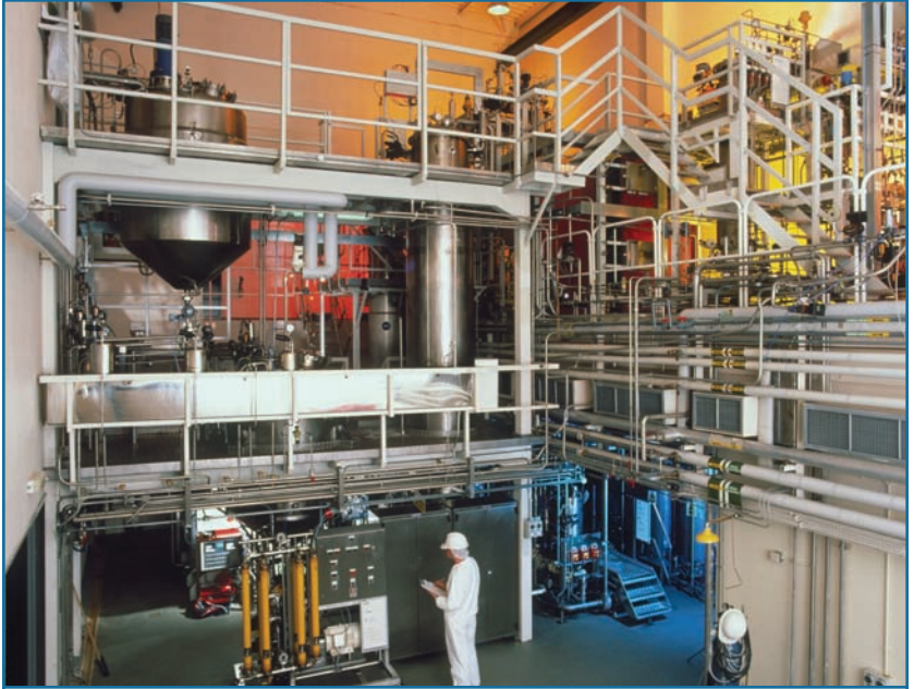
Figure 6.2 A large-scale fermenter used in the commercial production of monoclonal antibodies. © James Holmes/Cell Tech, Ltd./Photo Researchers, Inc.
